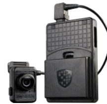
Digital Ally's FirstVU HD body camera uses a two-piece design to reduce the footprint and offer multiple mounting options. The camera head offers 720p HD resolution and a 95-degree angle horizontal field of view, captures HD audio, and is water resistant. (Image provided by Digital Ally)
